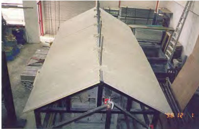
**Figure 3.** PSSDB folded roof structure tested by Ahmed (1999)
