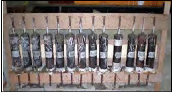
**Figure 5.** Casting of the specimens
