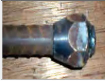
**Figure 4.** Tapered nut welded on steel bar
